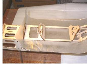
**3.6.10** Cut the canopy free afterwards. Find a 1/8 wooden dowel. Cut a 1/2 in. length from it, and glue it to canopy's C1b/C1x. Glue (Polyurethane glue or Epoxy) the included thumbtack at the hole on the slanted C4.
