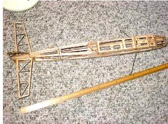
3.8.2 Test fit the whole wing assembly through the fuselage opening. Trim little by little until the wing comes to the right place. Align the wing from top view (equal distance to vertical fin) and rear view (parallel to horizontal stab.) Trim the opening more if necessary. If a gap becomes too big, you may use a stripe of balsa to shim the wing. **Recheck everything** before applying glue (Epoxy or Polyurethane.) (Note, more glue equals more weight. No need for excessive glue!)
