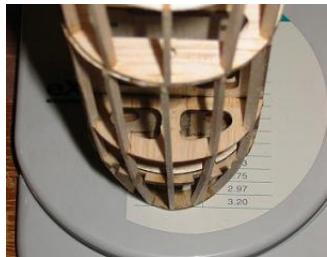
3.6.3 Cut and join two  $1/16 \times 1/8 \times 18$  sticks into one stick/stringer as shown. We need five long stringers for the lower deck.
