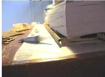
3.2.7 Remove phone books after a few hours. Fit and glue in all spar webs (VV-2). Note the orientation of those spar webs. The letter should be always on the lower and inner corner.
