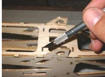
3.6.6 Install F7a, F8a, and F9a. Glue in vertical fin. **Check alignment of the vertical fin from review view and side view.**
