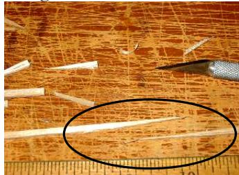
3.6.4 Install those five stringers on the bottom. The joints should be positioned roughly on F6. Trim the ends accordingly. . (**Φ:** After the glue dries, cut stringers to release the aileron service hatch.)
