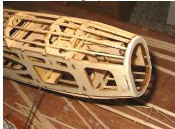
**3.6.12** Enlarge the hole on F6a. Fit and glue the included magnet in place. Use Epoxy or Polyurethane glue for this. The whole fuselage is now completed
