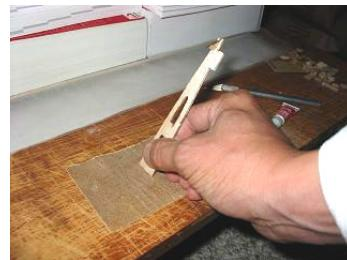
3.2.5 Under the main spar, place four pieces of 1/16 scraped balsa as shown. Fit center ribs and everything together. Fit W1 (ply). Use Ribs Jig to help alignment. Once everything lines up (double check!), carefully tack glue the whole wing together.
