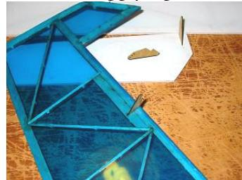
3.9.4 Refer to the plan, and install the tail wheel wire support (TB ply), then install small tube. Bend the remaining wire (~0.6 in) 90° as steering wire. Use Polyurethane or epoxy to attach the whole assembly to V10. Cut small piece of tape to hole the assembly on. Drill hole on rudder for steering wire. Install the rudder with tape on both sides as hinge.
