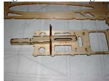
3.1.8 Glue F4a (ply) and F4b (1/16 balsa) together. Drill eight holes for landing gear tie wire. Place landing gear wire **on the side of F1a (ply)!** Twist the tie wire to hold down the landing gear wire. Cut and leave about  $\frac{1}{4}$ " to  $\frac{3}{8}$ " of twisted wire. Dab a little glue on the twist wires afterwards.
